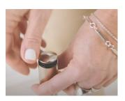
**2.** Press end caps into the outer edges of the closet rod.
