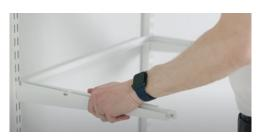
1. Begin at the left click-in bracket. Align the metal tabs on the gliding frame with the cutout notches of the click-in bracket. When aligned, press the gliding frame using your hand at the left rounded corner until you hear it lock into place.
